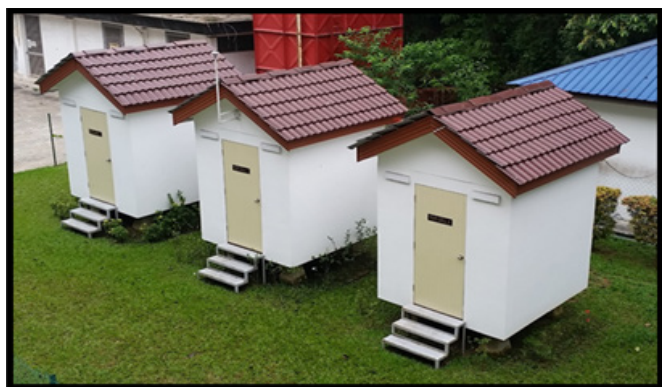
Figure 1 Photograph of small test units equipped for RSI measurement.
